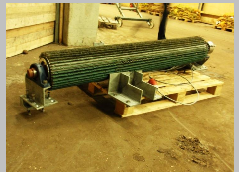
The Flex Trim sanding head is mounted under the dry roller supported by a girder made of iron.
