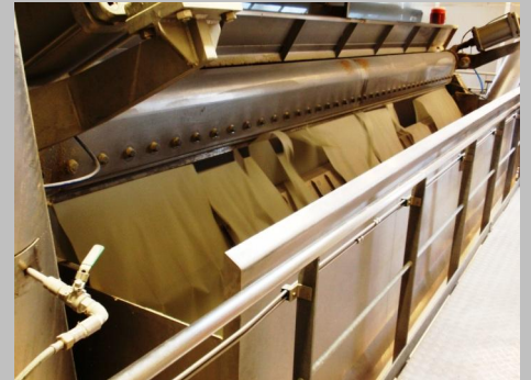
Potato turns to be dried flakes in the dry roller.
